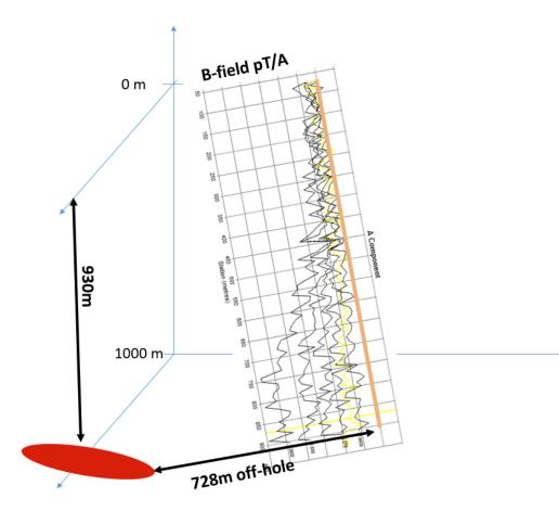
InfiniTEM<sup>®</sup> XL has 4 times more power than its predecessor InfiniTEM<sup>®</sup> Off-hole anomaly detected, 700 m off-hole at 950 m deep
